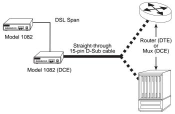
Figure 8. Connecting the Model 1082 to X.21 DTE or DCE
